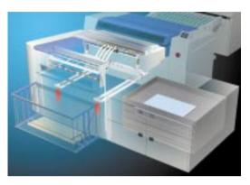
The lifting unit moves to the same level as the cassette that holds the selected plate type.
