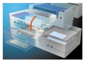
2 Suction pads grip the backside of the plate (no contact is made with the front) and it is loaded inside the PlateRite.
