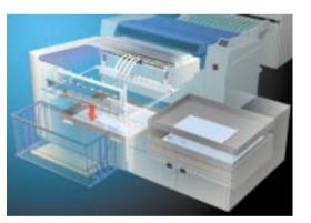
A sensor moves into place to detect whether the first layer is a plate or interleaf paper.
