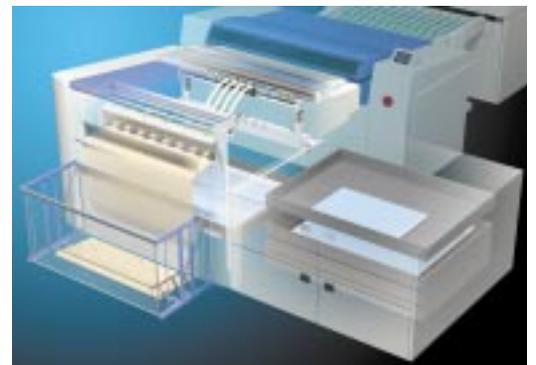
**4** The interleaf paper is lifted away and ejected to an external collection box.
