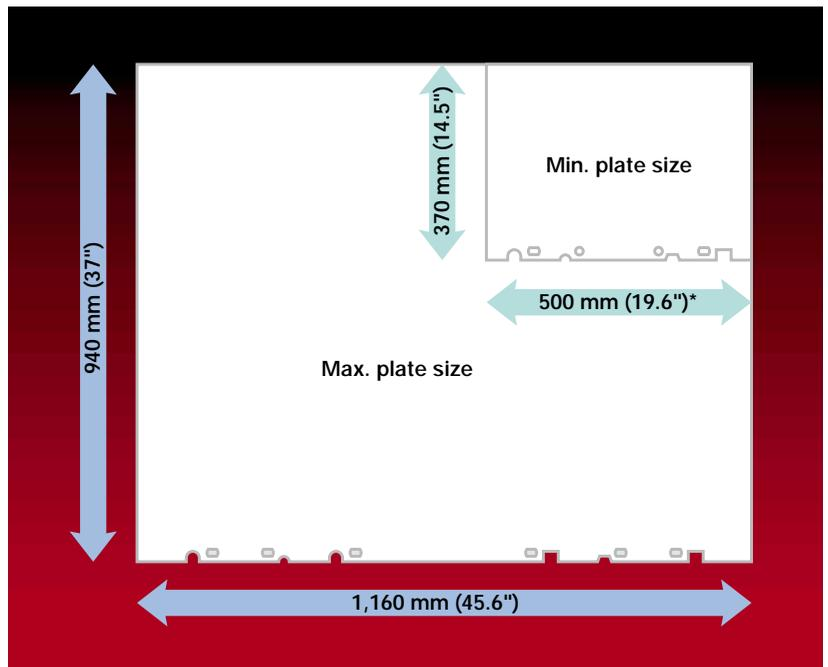
\* If manually loaded, even smaller plates can be used in the PlateRite 8000II. Minimum 450 x 370 mm (17.7" x 14.5").
