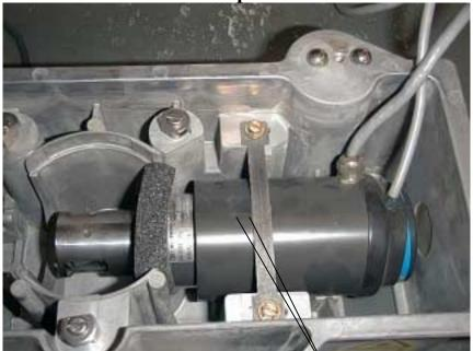
Take notice again of the scribe line on the motor with the notch on the metal strap, you will want to mark the ends of the metal strap with a pen so you are sure the metal strap gets put back to the original spot. Then remove the two gold screws and the metal strap.
