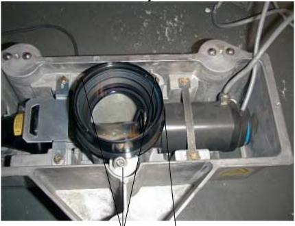
Turn the three quarter turn screws a half of turn to remove the 20-1 condense lens. This will give you access to the spin motor.
