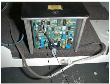
Remove these two connections from the LDM BD and gently slide the imager unit out the left side until the gray wires of the spin motor & fan become taut.
