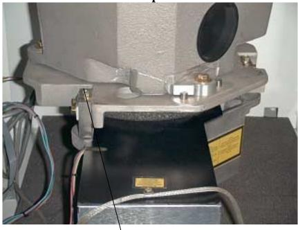
If facing the front of the machine this is a left side view. This is the second bolt that needs to be removed. The final bolt will be straight back behind the casting in front of you. The whole Imager unit will be lowered at this time.
