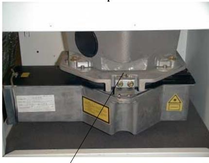
Loosen the three bolts from the top (this is a front view).
