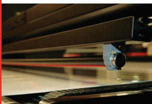
*Ionizer bar prevents anti-static loads*
